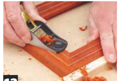
12 Clean up the surfaces with a finely-set block plane, but if timber has interlocking grain, then use a cabinet scraper for final smoothing
